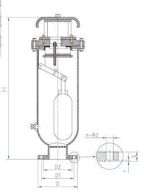
Class 300LB RF Flange dimension standard conforms as to: ASME B16.5
