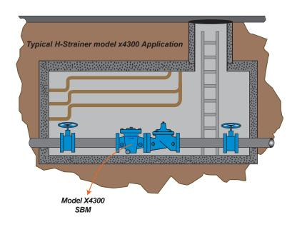
Because the Wye-Strainer prole extends below the pipeline, additional clearance is required to accommodate configuration as well as to allow for cleaning of strainer mesh.
