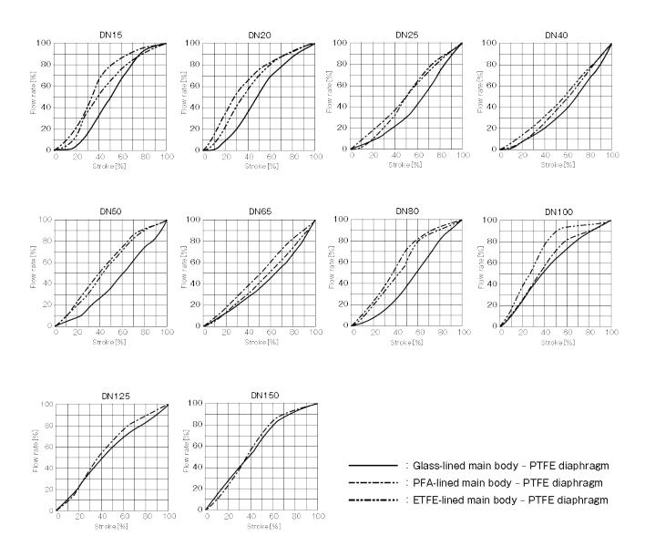
The charts show the specific flow rate characteristics actually observed by this company. In actual service, the flow rate characteristics may vary depending on the pressure, temperature, flow velocity, piping and other condition.
