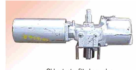
Old actuator fitted on valve
