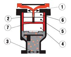
Disentrained air rises through the liquid and accumulates in the valve chamber. When the volume of air is sufficient to displace the liquid, float (4) will no longer be buoyant and will gravitate downwards thereby opening the small orifice (7) and allowing accumulat ed air to be discharged into atmosphere. As air is discharged the liquid raises the float (4) and re-seals the small orifice (7) and prevents the escape of liquid.
