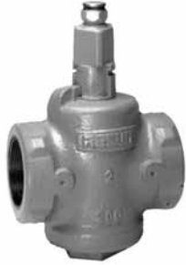
RECTANGULAR PORT THREADED Wrench and worm gear operated, regular opening and full pipe area, 1/2" to 4" sizes, 200 to 800 psi WOG.
