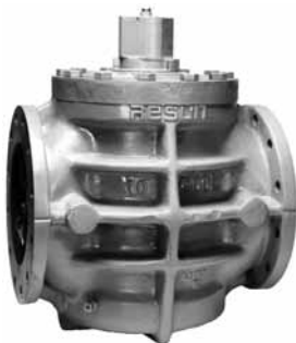
TOP-ENTRY CONSTRUCTION Bolted cover plate standard. Full pipe area: 200, 400 psi WOG: 8" size up- 500 psi WOG: 6" size up- Round Port: 5" size up-Venturi, 200, 400 psi WOG: 10" size up. Multi-port: 6" size up.
